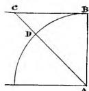
parts of this arc will be on a level. But a tangent BC meeting the vertical line AD in the point C will be the apparent level at the point B; and therefore DC is the difference between the apparent and true level at the point B.
